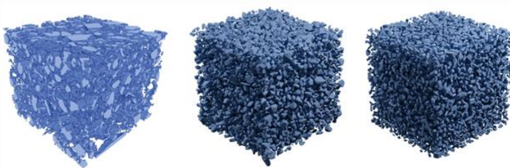
Figure 1: From left to right: an observation of a lithium sulfate coating, the polyhedral model, the simplified cuboid model.
