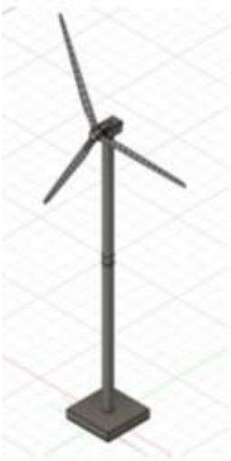
Fig. 1 The NREL 5-MW wind turbine scaled model
