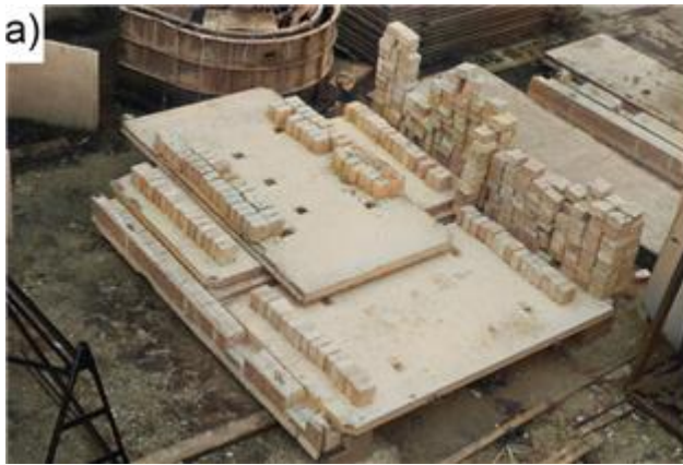
Test loads: a) view of floor slabs and concrete blocks loading the beam; b) view of load from masonry curtain wall
