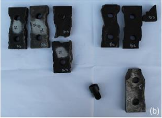
Fig. 2 (a) General aspect of the cutting assembly; (aa) conical shredding fittings, (ab) rectangular shaped cutting fittings, (b) fractured shear blades.
