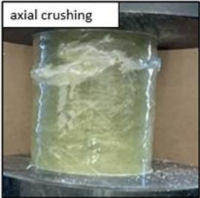
Lateral and axial crushing of GFRP and modified GFRP tubes
