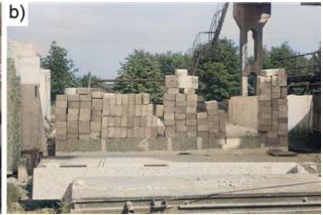
Test loads: a) view of floor slabs and concrete blocks loading the beam; b) view of load from masonry curtain wall
