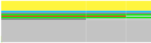
Fig. 2. Half the cross section of one cell from the considered CMUT device. The different layers are, from the top: the membrane (yellow), the additional membrane layer for the resonance frequency tuning (blue), the top electrode (light grey), the top passivation (green), the cavity (red), the bottom passivation (green), the bottom electrode (light grey), the substrate (light grey).
