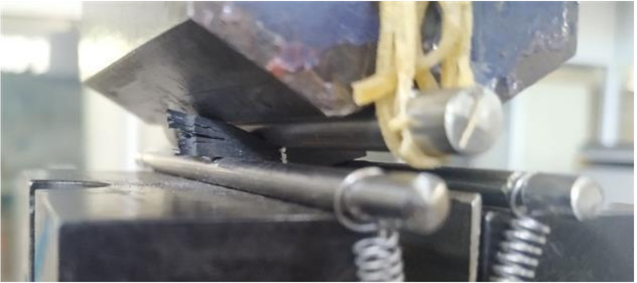
Short-beam Test (ILSS) of CFRP with CSR
