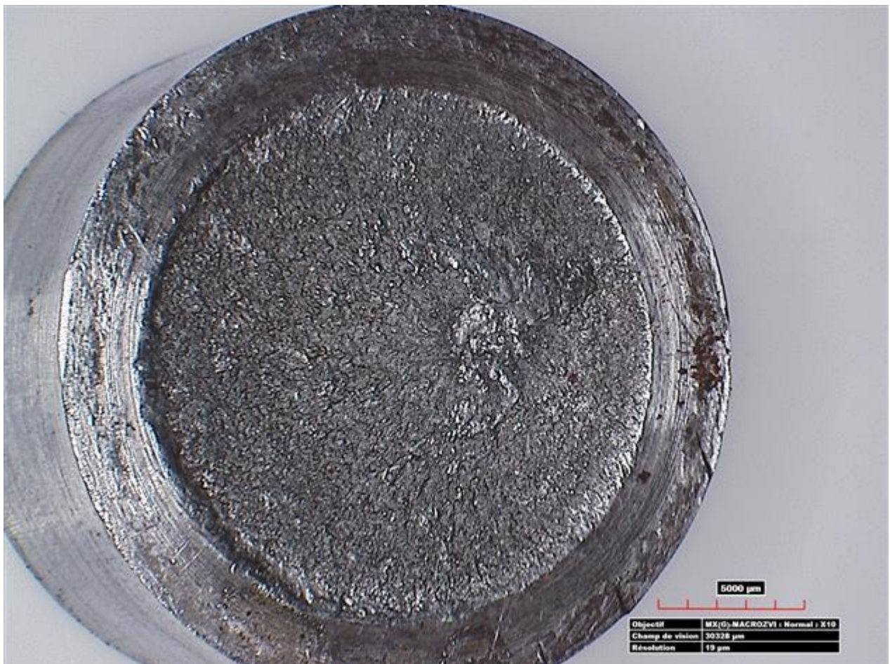
Figure 1. The broken rotating machine shaft.
