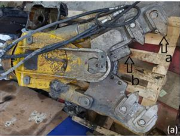
Fig. 2 (a) General aspect of the cutting assembly; (aa) conical shredding fittings, (ab) rectangular shaped cutting fittings, (b) fractured shear blades.
