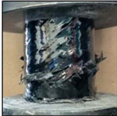
Lateral and axial crushing of GFRP and modified GFRP tubes
