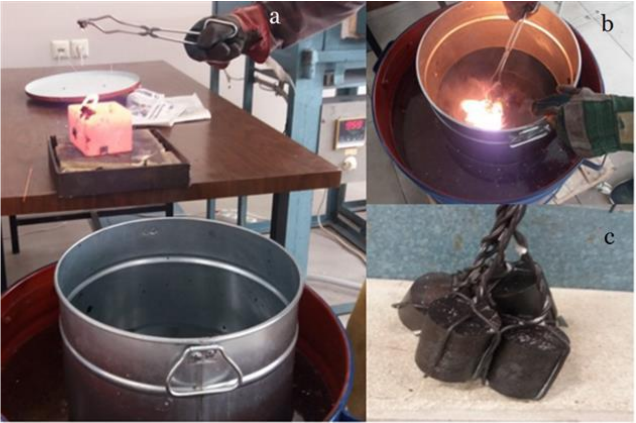
Images showing the oil quenching of samples.
