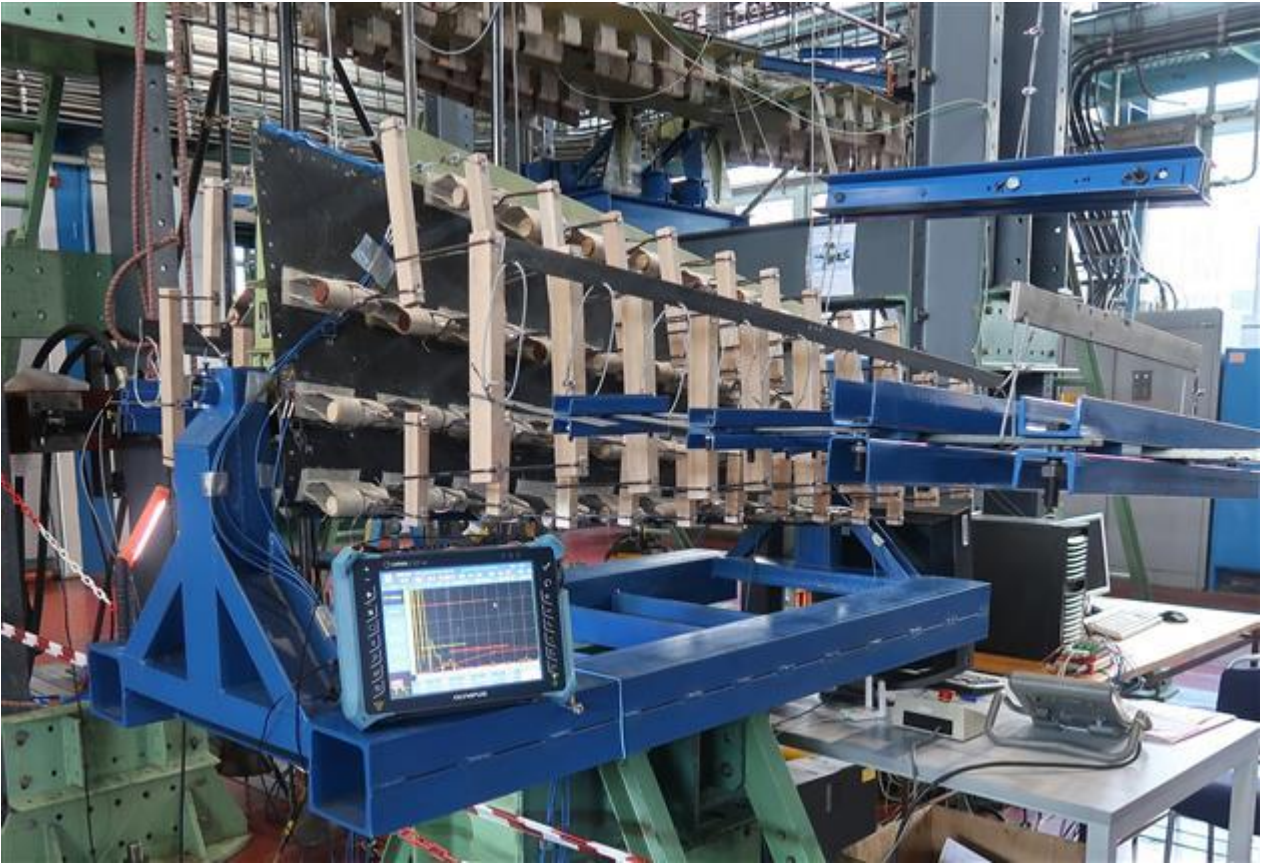
Fig. 1: NDT inspection during fatigue test of the aileron
