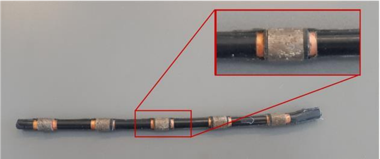
Section of a diamond wire with the representation of the portion to be modeled.
