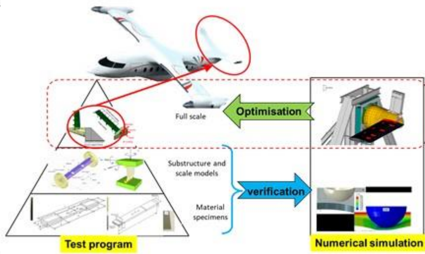
Building block diagram for testing and numerical simulation
