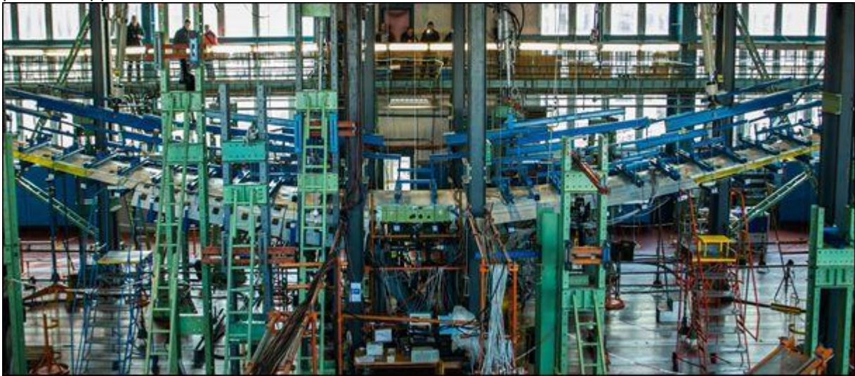
Figure 2: Example of test rig - Wing static test (national project) with simulation of variable stiffness of fuselage
